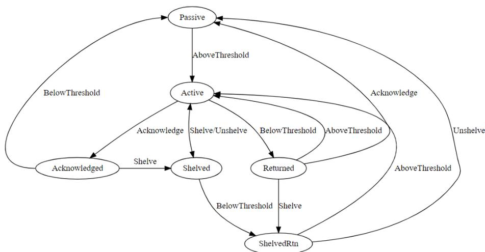
Figure 5-1: Alarm state diagram
