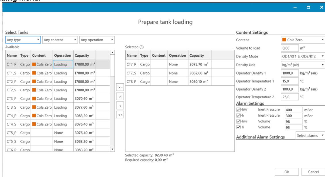
Figure 3-3: Prepare tanks for loading
