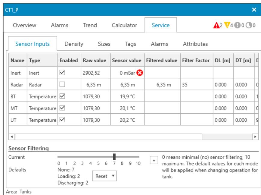
Figure 5-9: Disabling tank level radar
