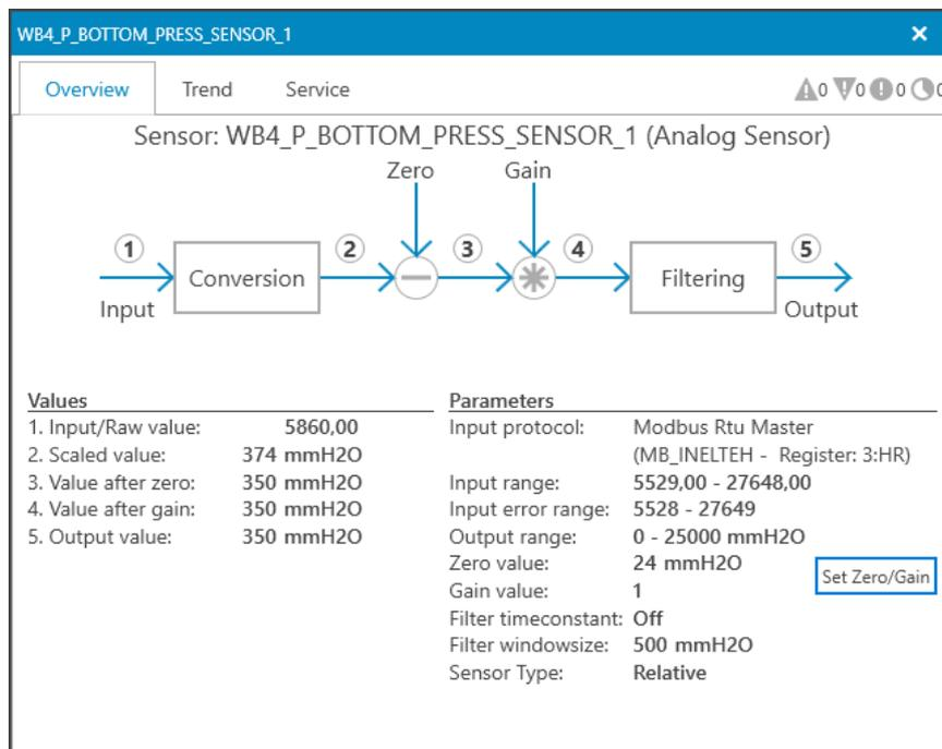
Figure 9-5: Sensor after zero (offset) adjustment
