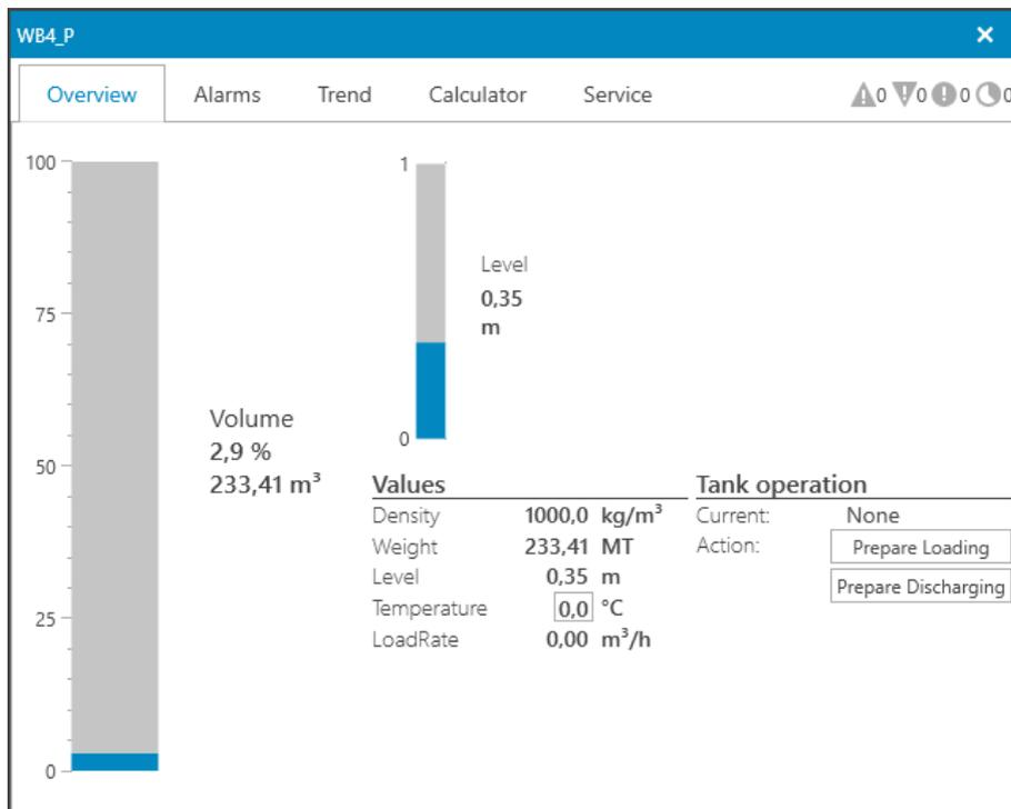
Figure 9-6: Tank after sensor zero (offset) adjustment
