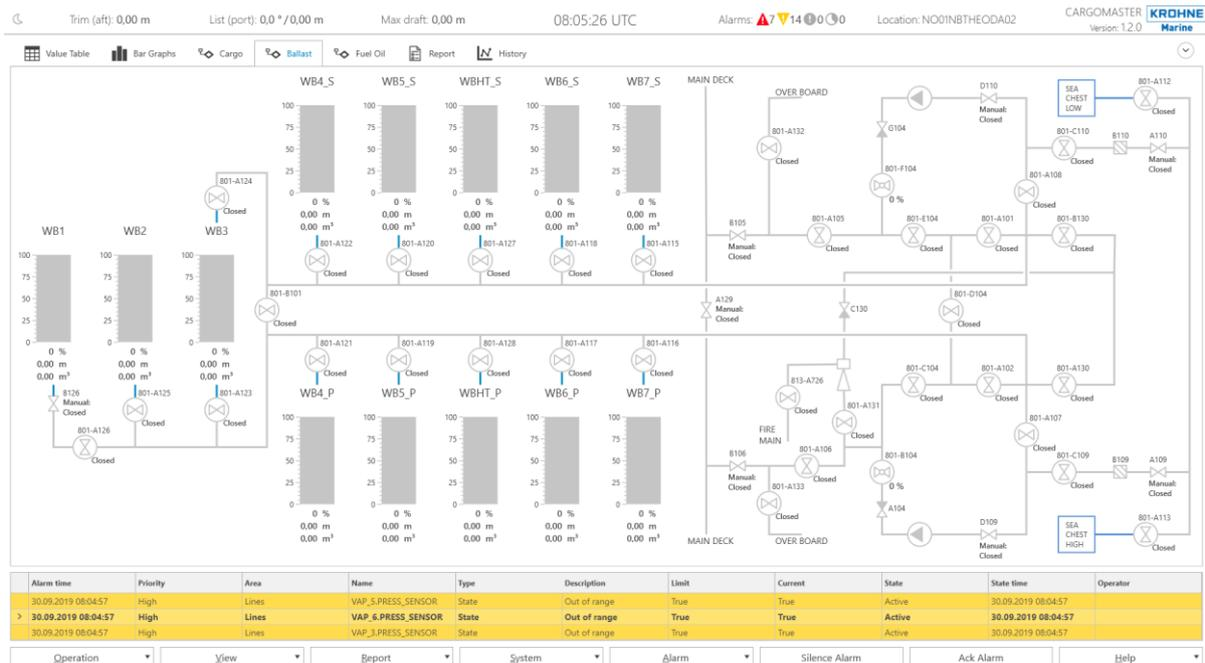
Figure 4-9: Ballast layout view
