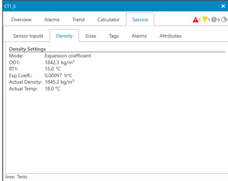
Figure 4-17: Tank faceplate - Density settings
