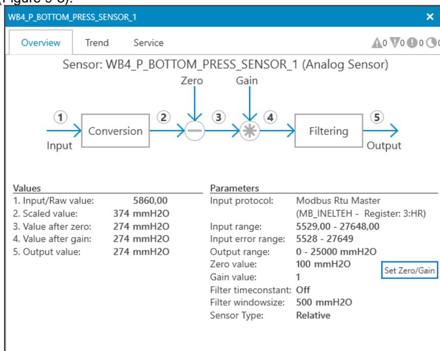
Figure 9-3: Analog sensor faceplate
