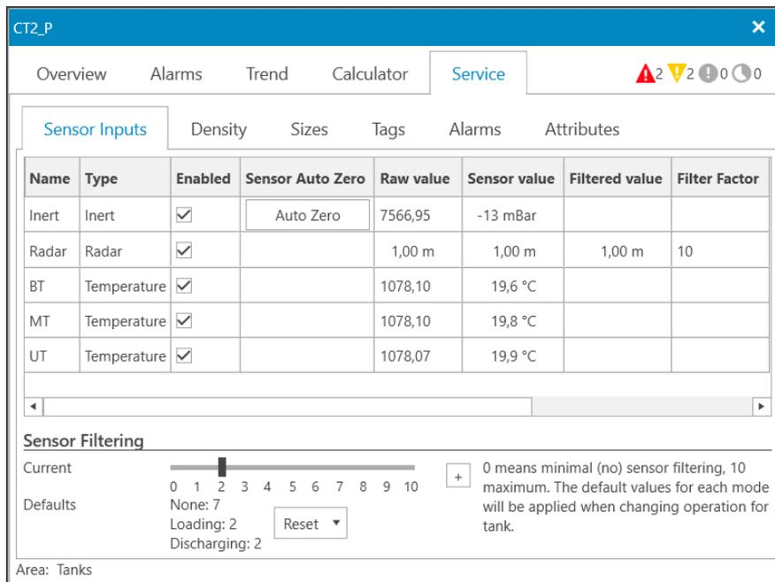
Figure 4-16: Tank faceplate - Service tab
