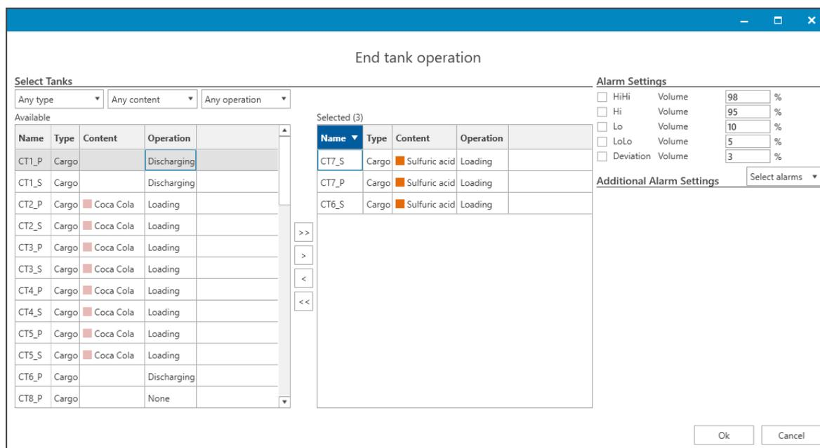
Figure 3-5: End operation on tanks
